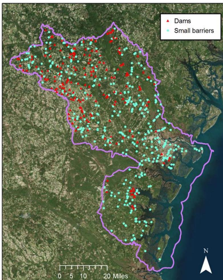
**Figure CS1-2.** Location of aquatic barriers within the Savannah River Watershed. Points representing where dams (triangles) or small barriers such as culverts (circles) exist.
