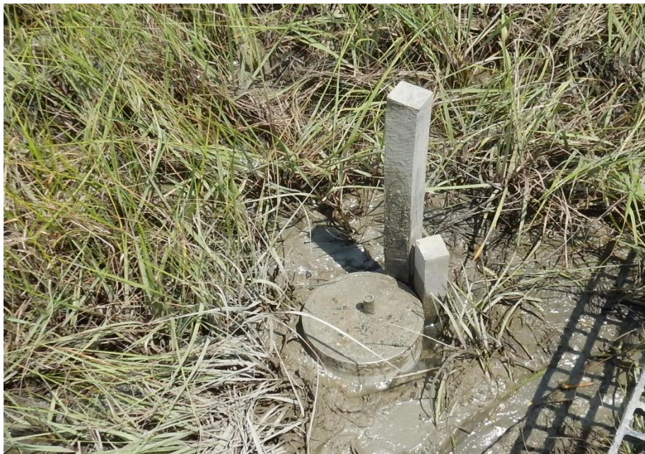
Figure 4: Rod with PVC "collar" filled with cement
