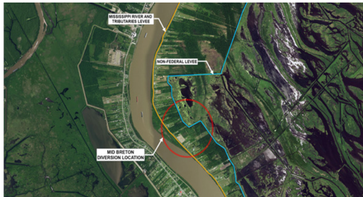
The proposed sediment diversion, above circled in red, will divert sediment and water from the Mississippi River into the Breton Sound Basin.
