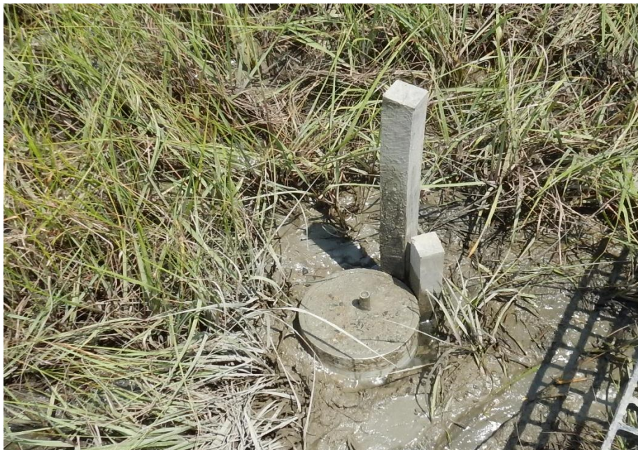
Figure 12: Rod with PVC "collar" filled with cement
