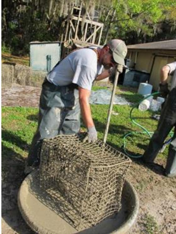
***Figure CS2-5. Gary Sundin of South Carolina Department of Natural Resources coating a crab trap with cement.***
