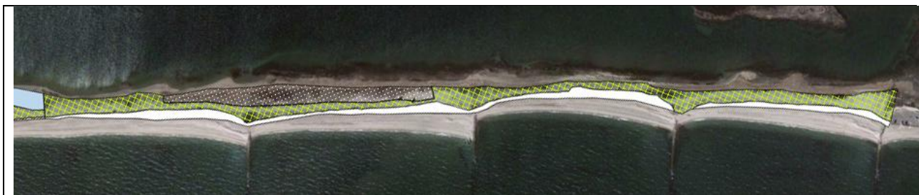
Figure 3. LBW landforms (top photo) include ridge plain (black lines), relict inlet dune (blue), berm (yellow) and eroded dune (white). Long Beach landforms (bottom photo) include primary dune (blue lines), eroded dunes (white) and backbarrier flats (cross hatch). Beach and tidal wetland are present in the imagery but not mapped.
