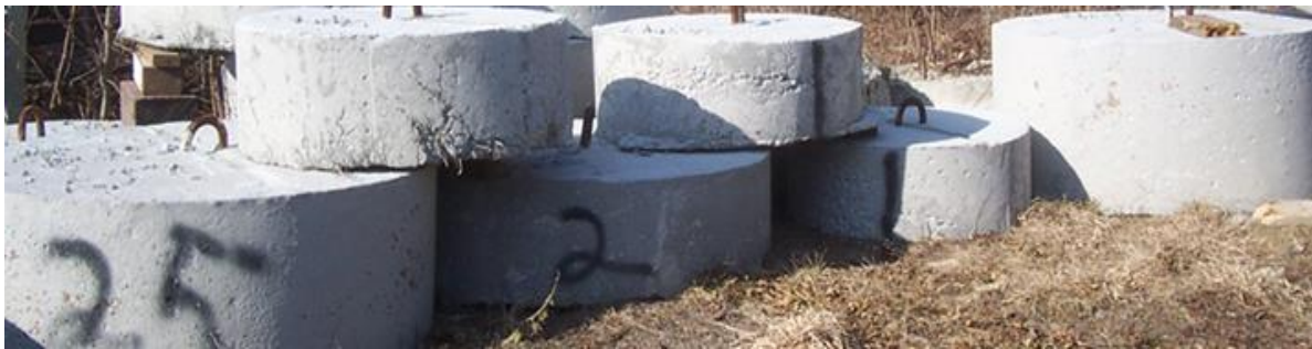
Figure 11. Deadweight anchors of poured concrete.
