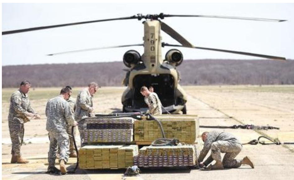
An air crew from the Connecticut Army National Guard's Bravo Company 2/104 Aviation Regiment rig three loads of lumber for lifting by one of the unit's CH-47G Chinook heavy-lift helicopters Friday at Groton-New London Airport in Groton. The lumber was bound for a U.S.
