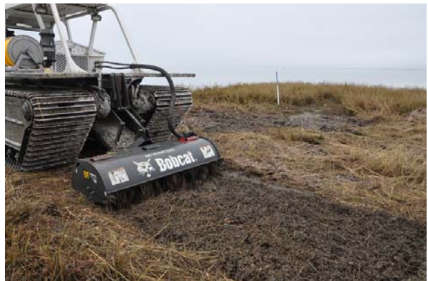
Above, marshmaster “swimming” to site (left), and with rototiller attachment following a top mow (right). Left, operator using a minitiller following top mow.
