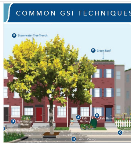
A screenshot of the City of Chester Green Stormwater Infrastructure Plan.
