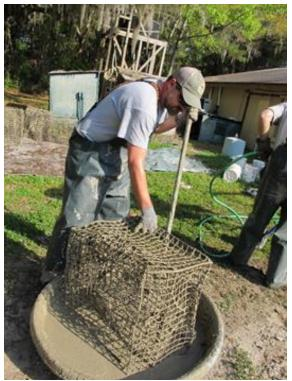
Figure CS2-5. Gary Sundin of South Carolina Department of Natural Resources coating a crab trap with cement.
