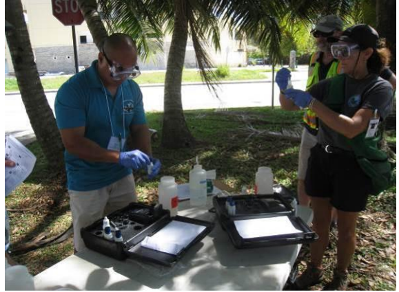
Use portable ammonia meters to test samples; ammonia may indicate sewage contamination.
