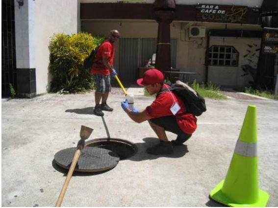
Collect a water sample from a storm sewer manhole to test for pollutants during an illicit discharge detection and elimination (IDDE) investigation.
